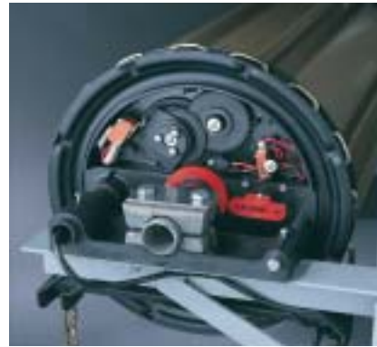
Detail A: End view of Drive Unit with access cover removed showing limit switches, cam gears and cut out switch. Also shown is the Manual emergency disconnect lever and the anchor block attached to wall bracket with dual anchor pins into the Drive Housing.
